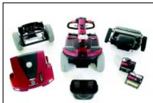
Easily disassembles into 7 components (Celebrity XL Deluxe shown above)
